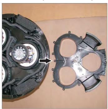
→ Remove the turbine casing.
